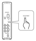
The Base Station is in setup mode, and the SETUP MODE LED on the front panel starts blinking in amber, and then lights.
